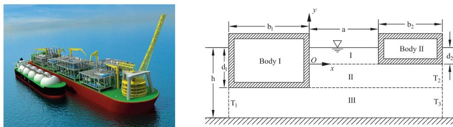
Figure 1: Side-by side offloading (Left). Sketch of the problem and coordinate system (Right).
