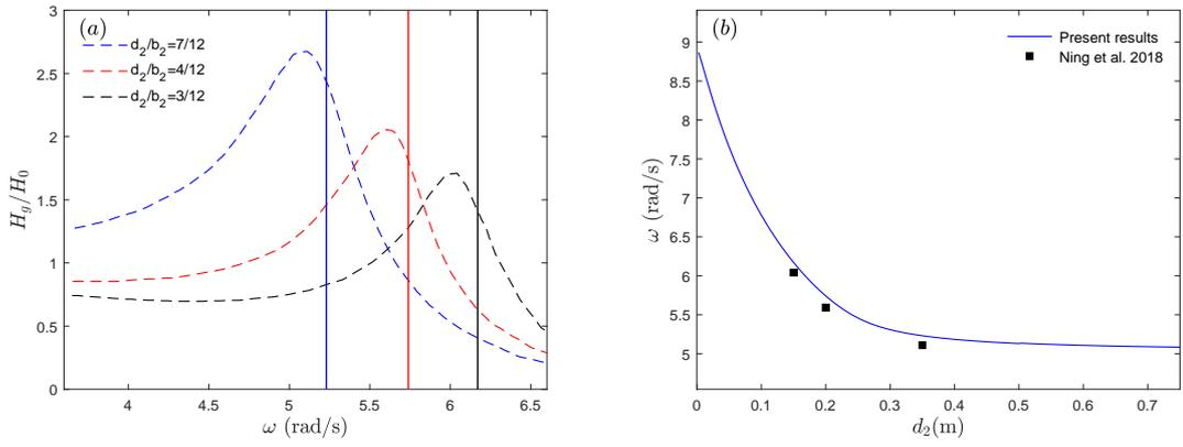
Figure 2: (a) Variation of wave elevation inside moonpool with respect to body draft  $d_2$  for  $b_1 = b_2 = 0.6$  m,  $a = 0.06$  m,  $d_1 = 5/12b_2$ ,  $h = 1$  m. The dashed line: results by Ning *et al.* (2018). The solid lines: present results on natural frequency (piston mode); (b) Variation of piston mode frequencies with respect to the draft of body II.
