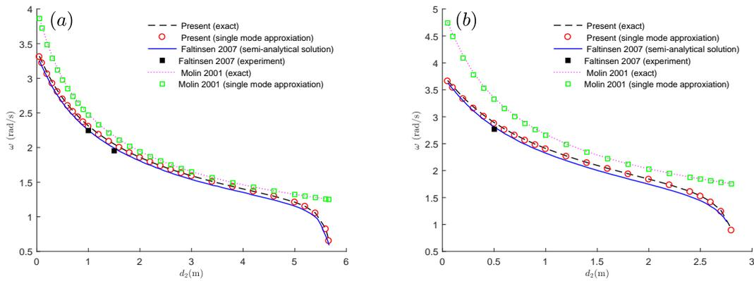
Figure 3: Comparison of the piston mode resonance frequencies with the experiments and other solutions. Variation of natural frequency with respect to the draft  $d_1 = d_2$ . Two cases are computed: (a)  $b_1 = b_2 = 2$  m,  $a = 1$  m,  $h = 5.72222$  m; (b)  $b_1 = b_2 = 1$  m,  $a = 1$  m,  $h = 2.86111$  m.
