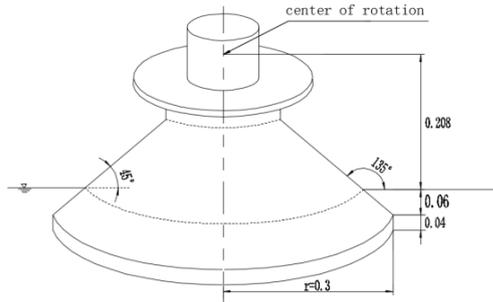
Fig.2 Cone-Shaped Floating Bodies
