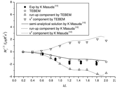
Fig.5 Second-order drift moments on Cone-Shaped Floating Bodies
