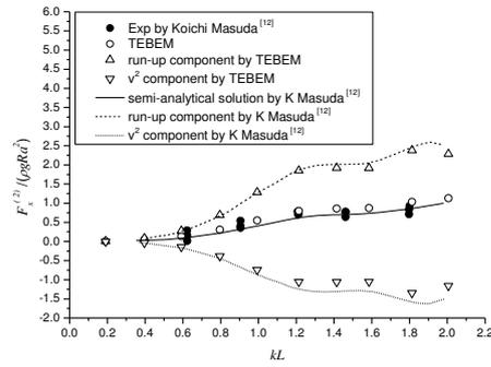
Fig.3 Second-order horizontal drift loads on Cone-Shaped Floating Bodies
