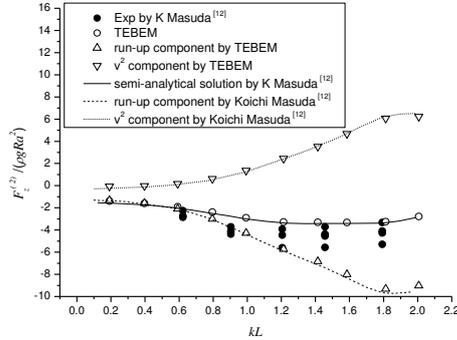
Fig.4 Second-order vertical drift loads on Cone-Shaped Floating Bodies
