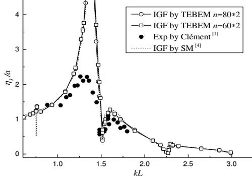
Fig.6 First-order heave response on box-shaped barge in wave tank with width 5.0m
