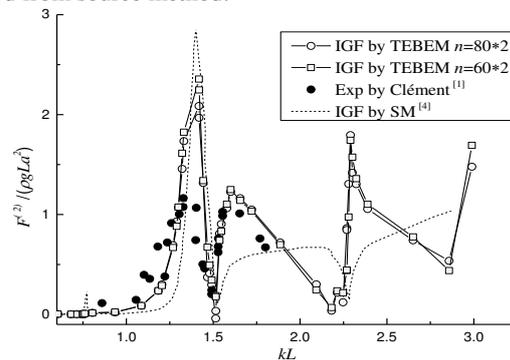
Fig.7 Second-order horizontal drift loads on box-shaped barge in wave tank with width 5.0m
