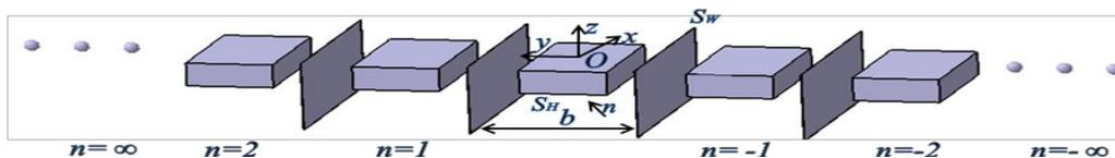
Fig.1 The sketch of side wall effects (four images)
